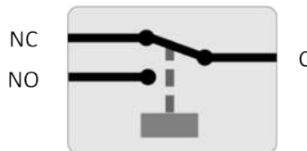
Internal operation of the programmable relay
