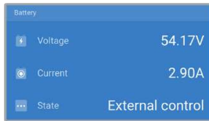
The VictronConnect app indicates that the charger is externally controlled.
