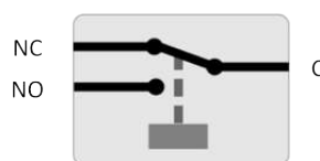
Relay configuration (not energised).
