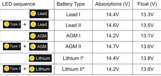
Lithium\* = live output voltage, ideal for waking up BMSs on batteries. Please ensure your lithium battery has an internal or external BMS. If you want a float voltage please use Lead or AGM profiles. If temperature sensor connected, no voltage compensation on lithium profiles. If temperature sensor detects 0 Deg C - BB stops charging.
