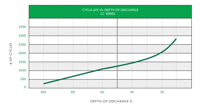
\* Cycle life may vary by application and is affected by frequency of cycling, operating temperature, depth of discharge (%DOD), adherence to manufacturer-recommended charging parameters and proper maintenance.
