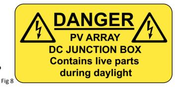
*Note: A PV system cannot be turned off – terminals will remain live at all times during daylight hours. It is important to ensure that anyone opening an enclosure is fully aware of this.*
