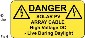
Where long cable runs are necessary (e.g. over 20m), labels should be fixed along the d.c. cables as follows:
