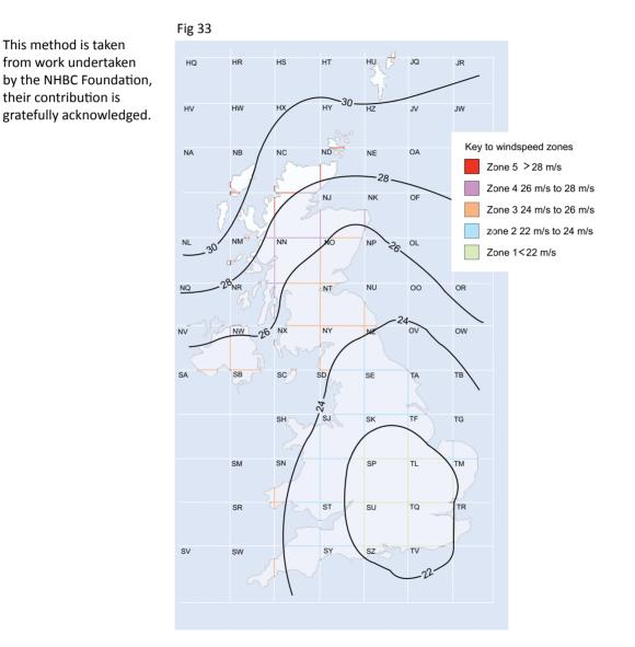
a. With reference to the site wind zone, site type (rural / urban), the ridge height of the building and the distance of the site from the sea - derive the peak velocity pressure  $(q_p)$  from the following table:
