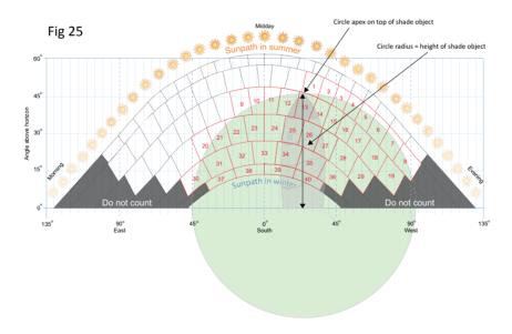
*Note:* The above diagram uses the same shade object as the worked example in section 3.7.7. Assuming the object is near shade results in a shade factor of 0.6 (compared with 0.89 in the previous calculation).
