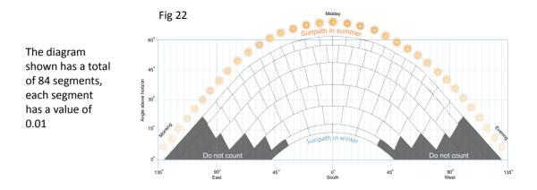
The sunpath diagram below shall be used to produce a shading analysis for all estimates produced.
