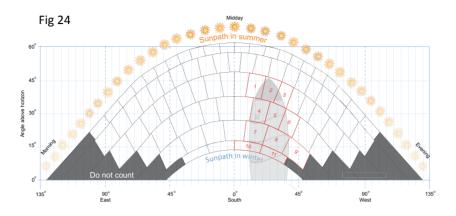
The total number of segments are multiplied by their value (0.01) and the total value shall be deducted from 1 to arrive at the shading factor.
